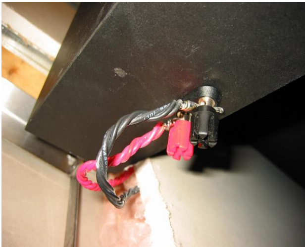
15. Attach the wires to the loudspeaker terminals. Be sure to observe the proper polarity! Tighten with large blade screwdriver.
