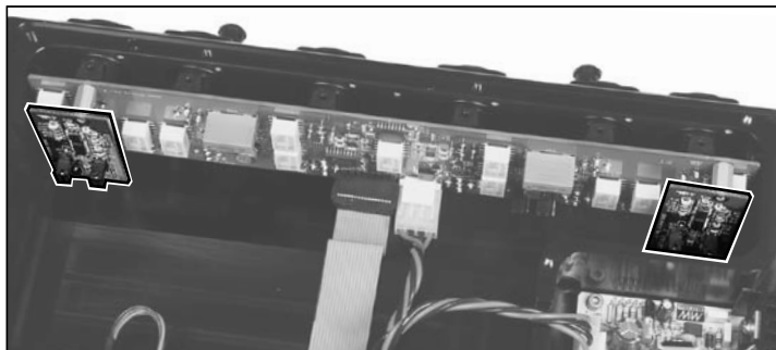
FIGURE 7: Location of both Phono Cards within the CONTINUUM chassis
